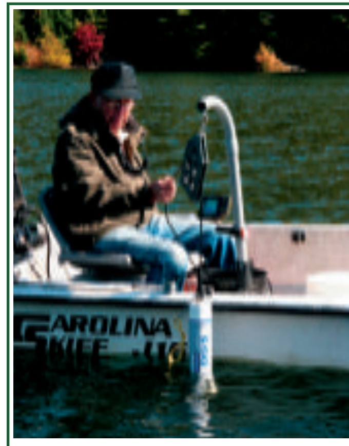
Don Henson on Lake Glenville collecting water samples with the sonde.
